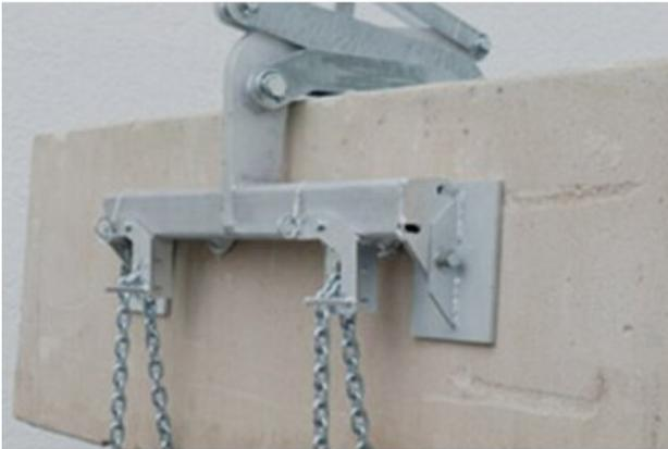
The galvanized wall panel lifting gear is used for the laying of horizontally positioned AAC wall panels. The profiled clamps ensure a high grip. If the safety chain is applied a transport high above the ground is permitted. The safety chain can be released by a tension rope of 10 m length.
