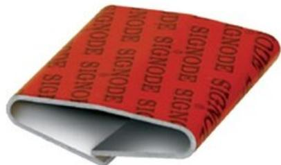
Ideal for round or irregular shaped bundles, push-type seals are used with a push-type tensioner to secure steel strapping. The flanges on a push-type seal completely overlap so both strap ends must be manually pre-threaded through the push seal before tensioning. These seals are usually crowned to prevent them from migrating too far into the hand tool during tensioning. A reverse notch joint is typically used to secure push-type seals.
