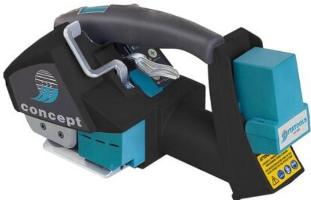
Automatic Tensioning Tool for Plastic straps is suitable for tensioning and cutting PET and PP straps. Tool clamps, locks and cut the plastic strap. The locking method uses friction welding.
