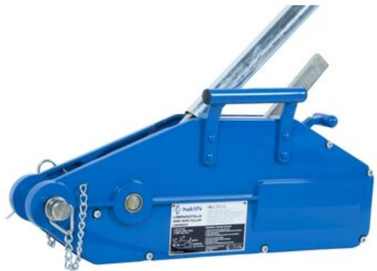
High quality aluminium wire rope hoist for pulling and lifting. The hoist does not have a wire drum as the wire goes through the hoist. Lifting and pulling speed is app. 3 m/min. The hoist is equipped with 20 m wire rope with a safety hook as a standard.
