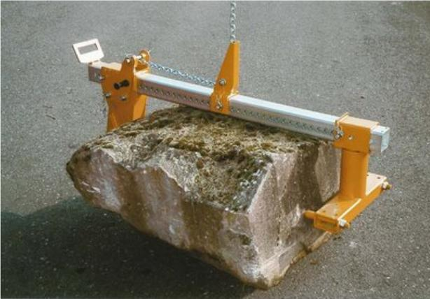
The boulder grab was developed for the simple transport of irregular stones and boulders. Of course, elements with parallel sides can also be transported.
